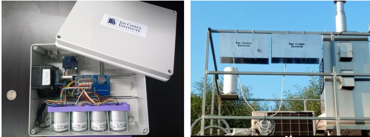
Figure 1: Picture of the low-cost Air Quality Monitoring system developed by researcher of the Cyprus Institute (left) and of the system installed at the DLI station (right).
